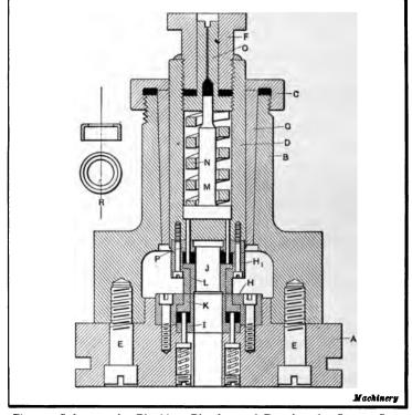
Fig. 4. Sub-press for Blanking, Piercing and Drawing the Copper Cup shown at  ${\cal R}$
